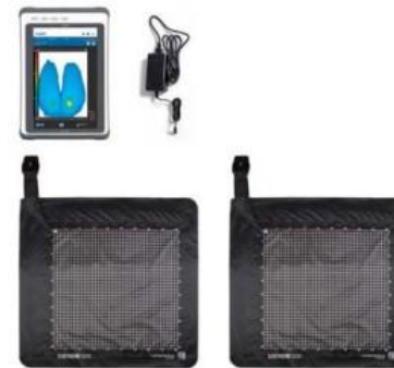
Pressure mapper (Rehab) used to determine areas of pressure for people in beds and wheelchairs
