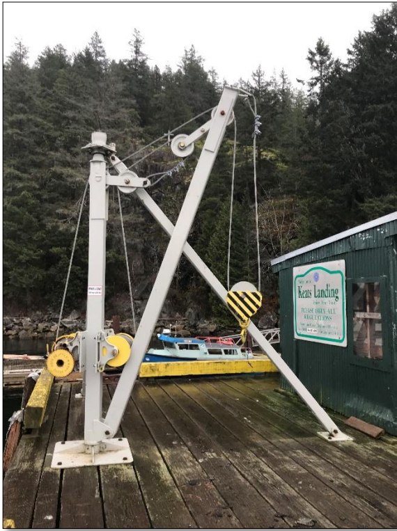
Photograph 11: Derrick crane, note: general arrangement
